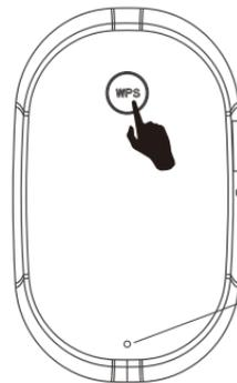
The LED should turn from blinking red to solid green, indicating a successful WPS connection. If not, please try METHOD TWO.
